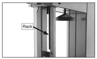
Figure 13. Rack lubrication location.
